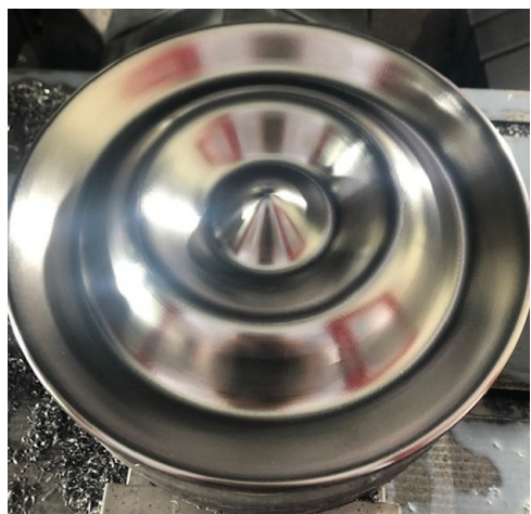
Surface finishing with more challenging cutting conditions
