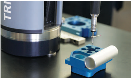
At only 13.5 kg, the C4 CNC accompanies you wherever you need it. No more need to bring parts to the CMM, the TRIMOS C4 can be implemented directly in production.
