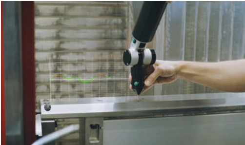
The new TRIMOS A3 measuring arms ensure extremely easy and precise 3D measurement. Certified according to ISO10360-2 or ISO10360-12, they allow quality control, inspection and inspection of medium and large parts.
