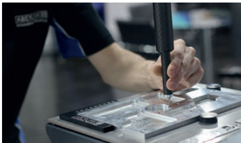
Magnetic jigs allow the workpiece to be clamped quickly, ensuring that all points are precisely measured.
