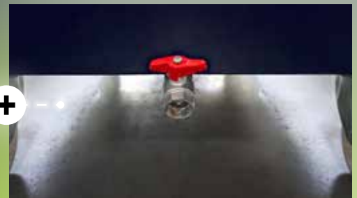
Watertight collection tank with sheet metal filter for the separation of liquids and solids and ball drain cock.
